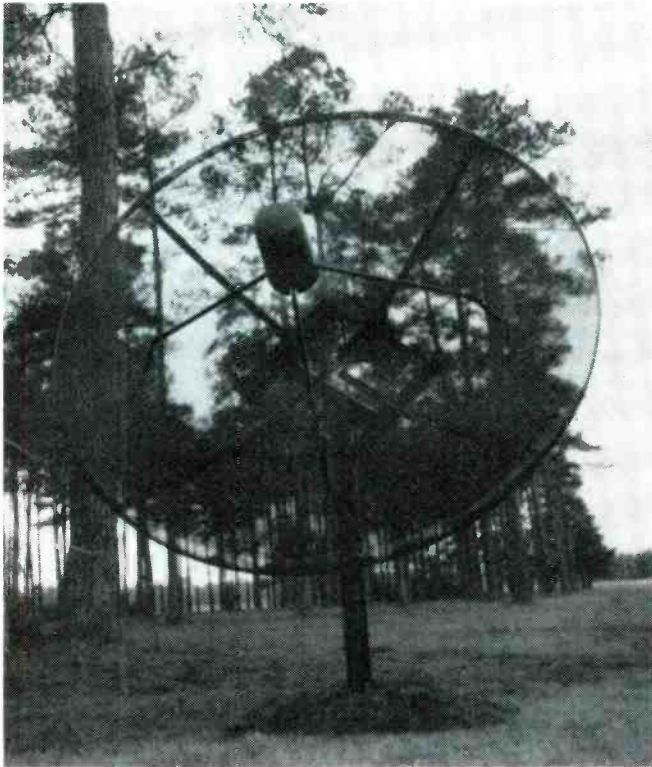
The 16-foot, parabolic-dish antenna from Birdview on the right, coupled with a block downconverter can feed satellite-TV signals to a multi-unit apartment complex. The dish is the one component in a satellite system most responsible for good or poor reception. As a rule of thumb, however, 10- to 12-foot dishes are generally of sufficient size for most parts of the United States. Although the solid Fiberglass parabolic dish is more commonly used, the open mesh type, constructed of spun aluminum, like the one from Channel Master on the left, offers less wind-loading.
