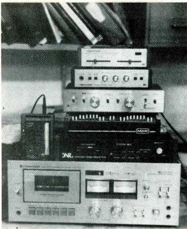
The author's system for improving noisy monophonic tape recordings which were made years ago. The video sound processor functions as in Figure 1. Bass is added by the bass enhancer on top. Body (full concert hall sound) is added with a small amount of reverberation. A graphic equalizer changes frequency response to fit taste. A second stage of DNR is sometimes used.
