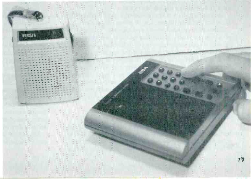
Fig. 5—The infrared transmitter may be tested by placing it next to a portable radio. Turn the volume of the radio fully on, set tuning dial below 530 kHz (bottom of the dial). Place the end of the remote transmitter close to antenna and press the control buttons. A gurgling or chirping noise indicates that the remote transmitter is functioning normally.
