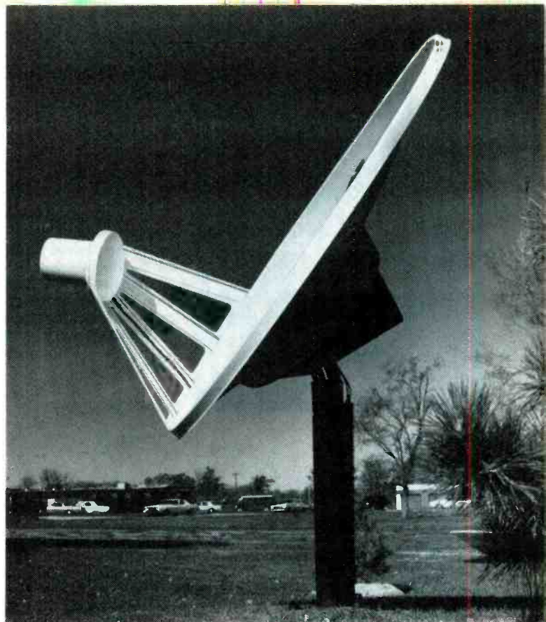
The 16-foot, parabolic-dish antenna from Birdview on the right, coupled with a block downconverter can feed satellite-TV signals to a multi-unit apartment complex. The dish is the one component in a satellite system most responsible for good or poor reception. As a rule of thumb, however, 10- to 12-foot dishes are generally of sufficient size for most parts of the United States. Although the solid Fiberglass parabolic dish is more commonly used, the open mesh type, constructed of spun aluminum, like the one from Channel Master on the left, offers less wind-loading.
